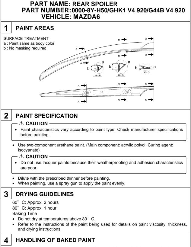
After baking, do not touch the painted product until it has cooled down completely.
