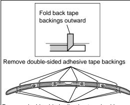
Remove double-sided adhesive tape backings
